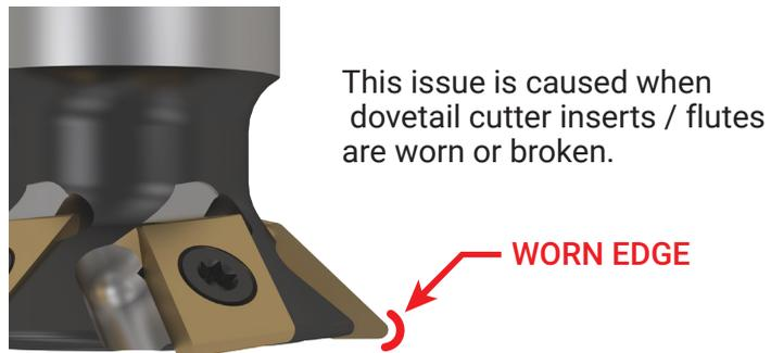
This issue is caused when dovetail cutter inserts / flutes are worn or broken.
