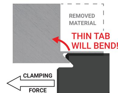
A thin tab and/or insufficient material on the top locating surface will allow the part to move during machining.
