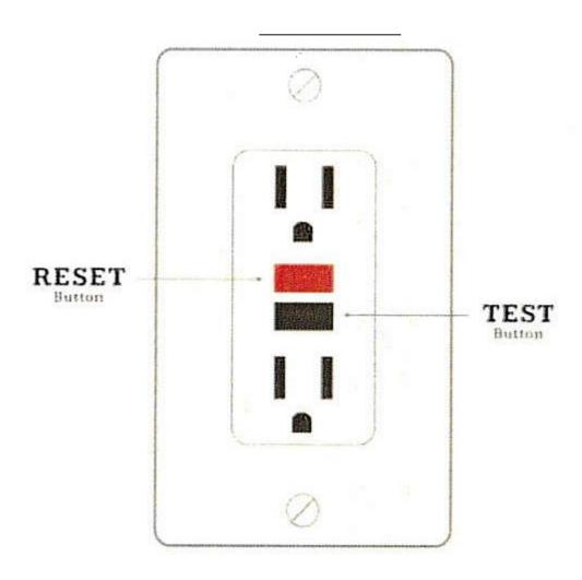
Above is an example of a GFI outlet. The buttons are labeled RESET and TEST.
