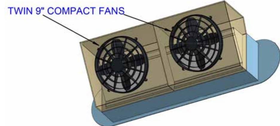
Vessel cut out (penetration) size = 700mm Wide x 180mm High
