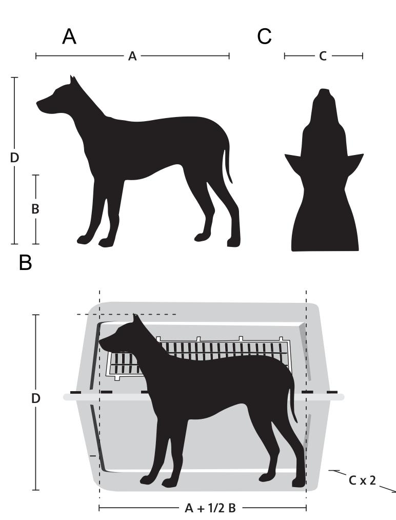
Minimal INTERIOR container dimensions: Length = A + 1/2 B Width =  $C \times 2$  Height = D
