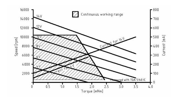
Sensorless commutation – Conform to industry standard 60° electrical. Motor using sensorless drive technology, to be used in combination with back-EMF commutating motor-IC (likes Philips TDA 51... family)
