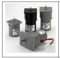
The Premotec Iron core motors have a modular structure that allows the motor to be integrated with two gearbox types in ratios from 6 to 729:1. The use of plastic in these motors minimizes cost whilst giving high resistance to chemicals and corrosion. Reliability is maximized by using internal spark suppression. Metal-geared versions are available for higher torque versions. Below is a list of our iron core motor program.
