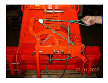
You are able to test the correct clutch adjustment, by checking the weight of the pull to activate the green cord – make sure the clutch arm is pulled all the way to the welded stop each time.
