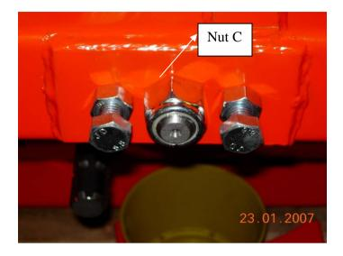
Loosen the two clutch adjustment bolts (Bolt B).
