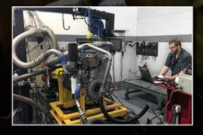
Live-run, computer-assisted dynamometer testing of Running Complete Diesels ensures trouble-free performance. Using the latest scan tools, JASPER tests engines under varying loads to simulate inthe-vehicle operation. Testing is concluded with a final engine run-in and inspection to ensure peak performance and operating efficiency.
