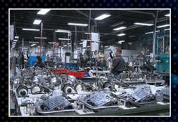
IASPER Transmissions are remanufactured in cellular environments known as PODs. These teams specialize in a specific transmission or a family of transmissions. This approach allows for cross training and has improved the quality and efficiency of our operations to hold the line on costs and increase the availability of our transmissions for you and your customers.
