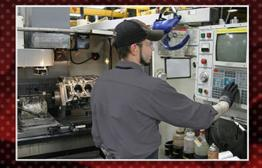
The latest Computer Numerical Control (CNC) machinery provides the versatility of resurfacing an engine block and boring its cylinders where applicable. Improved probing and tooling features provide optimal machining accuracy and surface finish.
