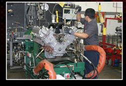
Most popular complete gas engines are live-run tested with data acquisition. Compression, vacuum and oil pressure are monitored and recorded. Testing is concluded with a black light leak inspection to ensure engines are free of oil leaks.
