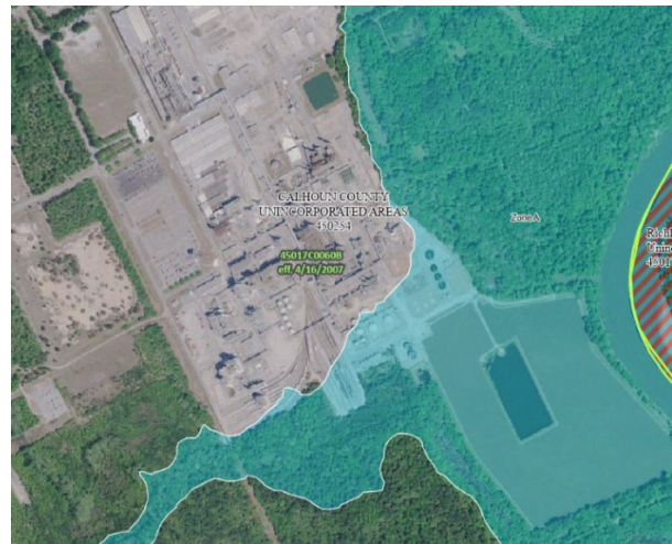
Figures 9 & 10. The components of the wastewater treatment system at the Columbia Plant (left), overlaid with FEMA's 100-year floodplain layer in teal (above).
