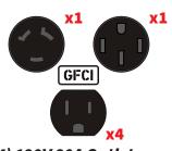
(4) 120V 20A Outlets (1)120V/240V 50A Twist-Lock (1)120V/240V 30A Outlet
