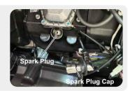
2. Unscrew the spark plug from the generator using the spark plug wrench included with this product.
