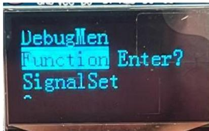
3. After pushing SET button to enter, there will be a prompt for the password. The factory default password is "006". Push the SET button to enter the password. The password may be changed to another 3-digit number in the configuration menu if required. In this photo, the password has been changed to "000".
