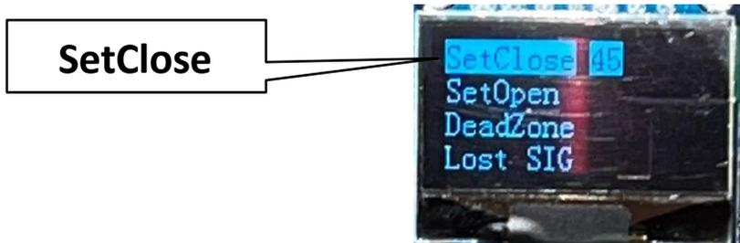
6. The CLOSE and OPEN positions are set according to the position of the 0-1000 Ohm potentiometer output resistance values (ohms) corresponding to the actuator rotation (in degrees) from the chart below:
