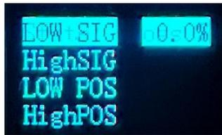
7. To calibrate the Low Signal, push SET button
