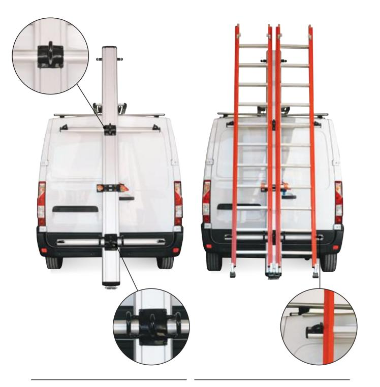
Two ladders can be mounted side by side. Two adjustable ladder retainers ensure that the ladders are held in place during transit. Securing straps hold the ladders firmly against the ladder rack at all times.
