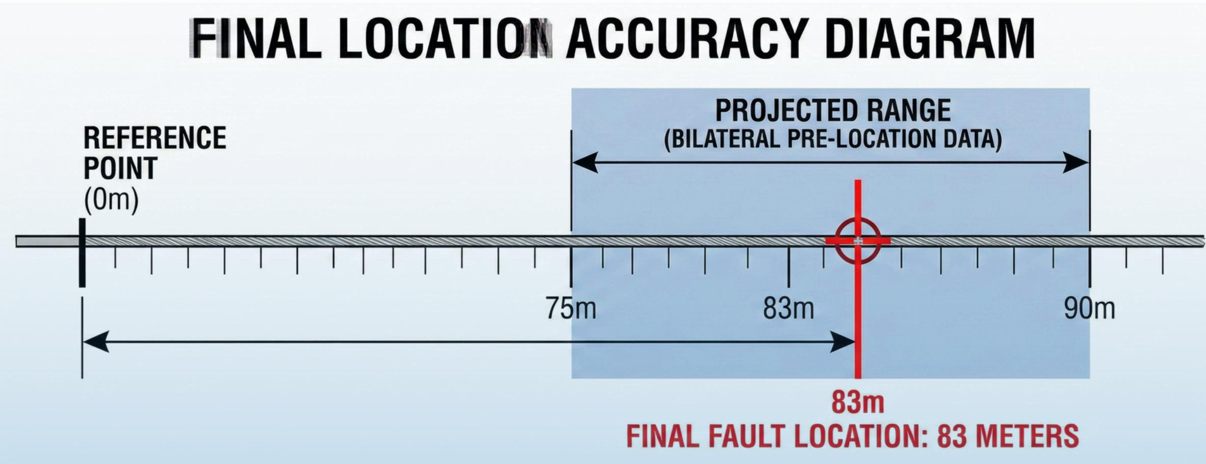
The final fault location was found at 83 meters from the reference point, a distance falling precisely within the projected range established by the bilateral pre-location data.
