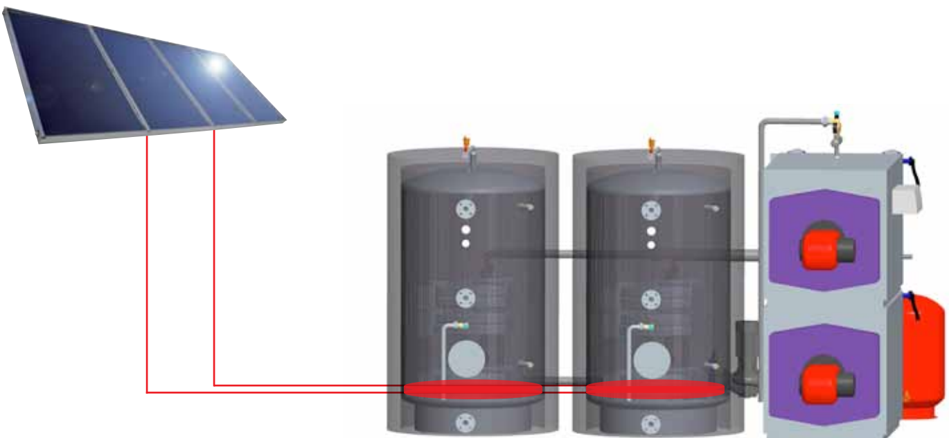
Schematic drawing how to include a solar system at the Smart Hot Water & Boiler Packages of type EWBI-EHSF.
