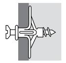
Pre-drill and insert anchor into hole.
