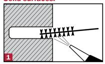
Drill correct size hole and clean out drill dust
