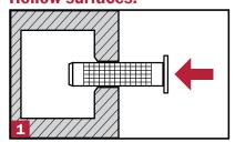
Drill correct size hole and insert screen brush
