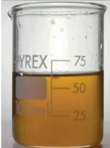
DIESEL BUG SUSPENDED IN THE FUEL
