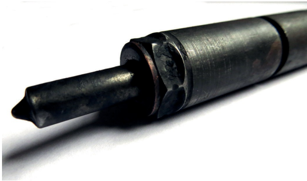
Injector before use of HC24
