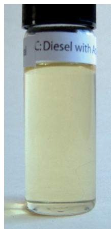
Non agricultural diesel plus 10% water treated with HC24™
