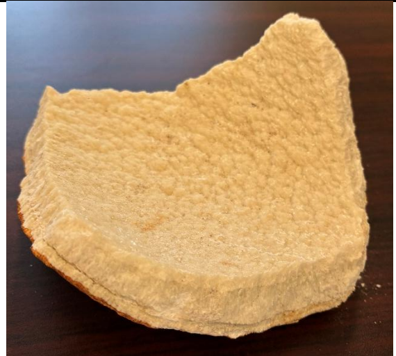
Calcium carbonate removed during recent cleaning at Keating Well WTP
