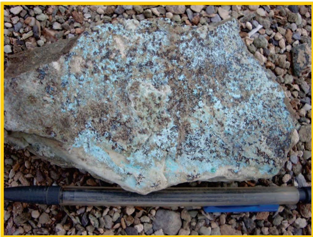
Figure 9b. Chrysocolla ( $(\text{Cu}, \text{Al})_2\text{H}_2\text{Si}_2\text{O}_5(\text{OH})_4 \cdot n\text{H}_2\text{O}$ ) with various Mn-Cu oxides in a Samalayuca sandstone bed.
