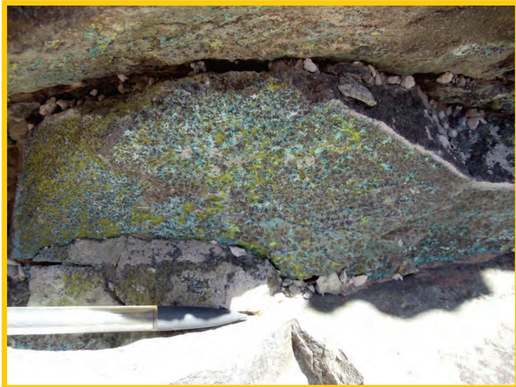
Figure 11a. Volborthite ( $\text{Cu}_3\text{V}_2\text{O}_7(\text{OH})_2 \cdot 2\text{H}_2\text{O}$ ) a brownish green V-Cu-bearing mineral accompanied by chrysocolla ( $\text{Cu},\text{Al})_2\text{H}_2\text{Si}_2\text{O}_5(\text{OH})_4 \cdot n\text{H}_2\text{O}$ ).
