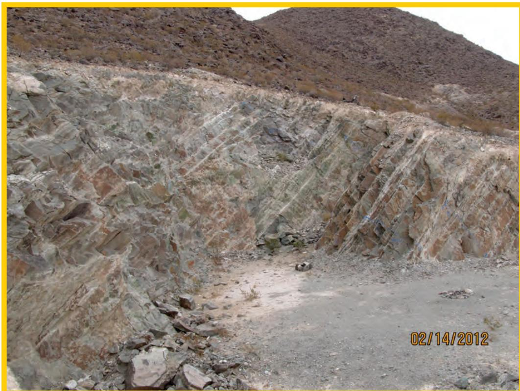
Figure 8a. Typical green (chloritized) sandstone beds interlayered with shale. Concha open pit.
