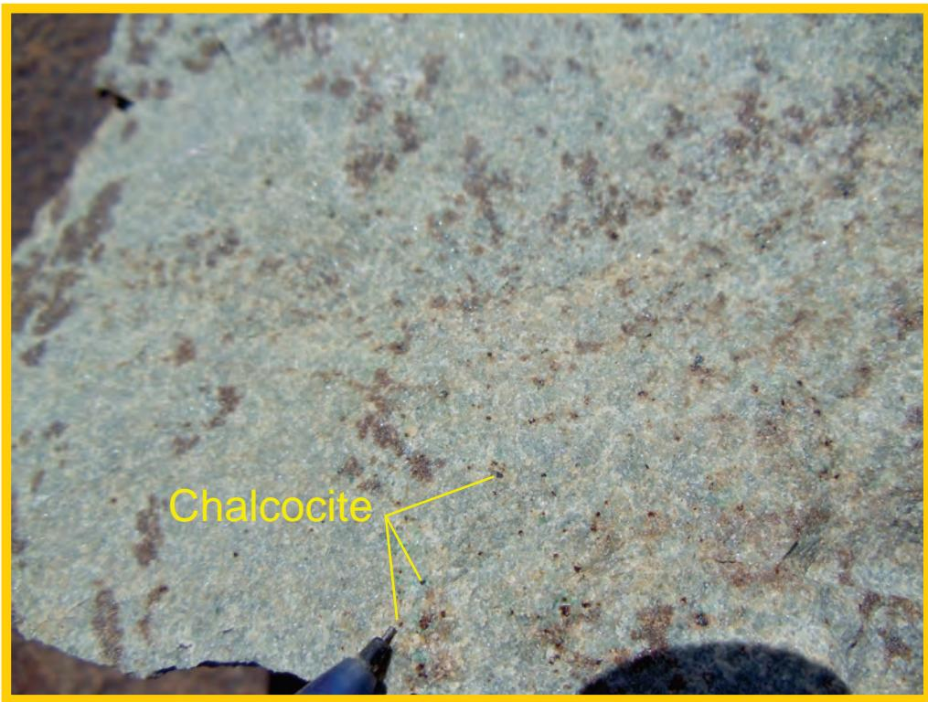
Figure 9a. Grains of supergene (?) calcocite ( $\text{Cu}_2\text{S}$ ) in a Samalayuca sandstone bed.
