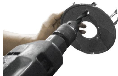
6. Drill a hole for Dia. 12mm.
