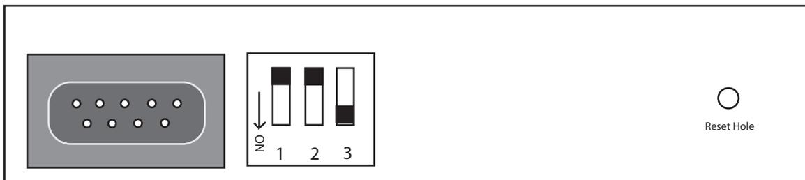
Dip Switch 3 is in the Down/ON position. Use this setting when connecting the RCV-5000 to a host PC for programming. Dip 3 must be turned ON (Down) before the RCV-5000 program auto-scan will recognize the RCV-5000. Once programming is complete, move Dip 3 to the UP/OFF position.
