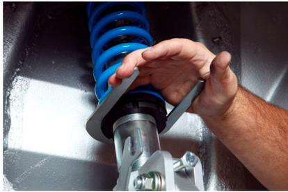
13. Slide disc onto bearing hub. Pull into position evenly with nuts and washers (not supplied)
