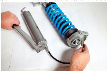
6. Grease the top bearing with chassis grease prior to install
