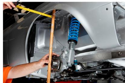
12. Adjust spring tension to desired feel and final height requirements and securely lock the 2 x spring settings
