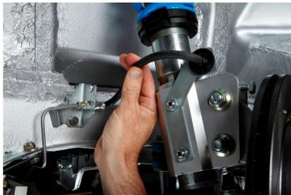
22. Fit the new tie rod or tie rod adaptor sleeve, supplied with the RRS kit, counting the same number of turns as the old tie rod end into the rod end adjuster sleeve
