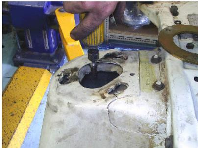
3. If your vehicle is a '65 -'73 Mustang, '66 Falcon, Fairlane etc. it will require 3 holes to be drilled through the original spring seat. These holes should be positioned directly under the original coach bolt
