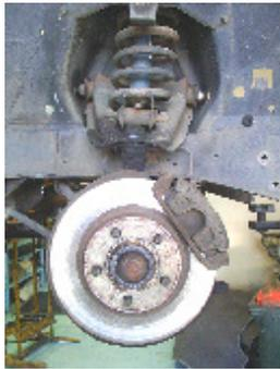
2. Some of the original Ford upper spring seat pressings may have deformities that may need dressing with a hand disc grinder or die grinder to allow an interference free fitting of the RRS upper mounting plate
