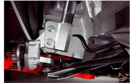
9. Connect the steering knuckle to the lower ball joint, tighten ball joint nut and split pin
