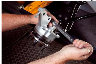
10. With a jack under the lower control arm, lift the steering knuckle high enough to connect the strut leg with the two large nuts and bolts supplied
