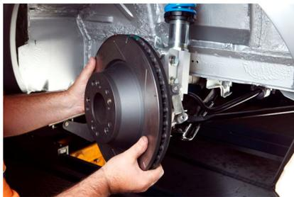
14. Warning: Do not over-tighten nuts to avoid stud or disc damage, however make sure that disc is fully seated on bearing hub otherwise calliper misalignment will occur
