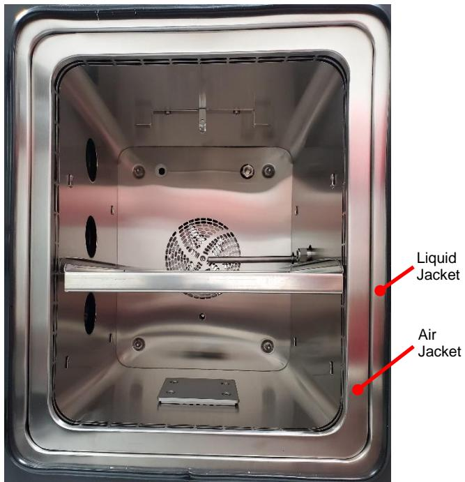
silicone profile seal for perfect tightness. An integrated chamber fan provides internal air circulation which ensures uniformity and stability throughout the working volume.
