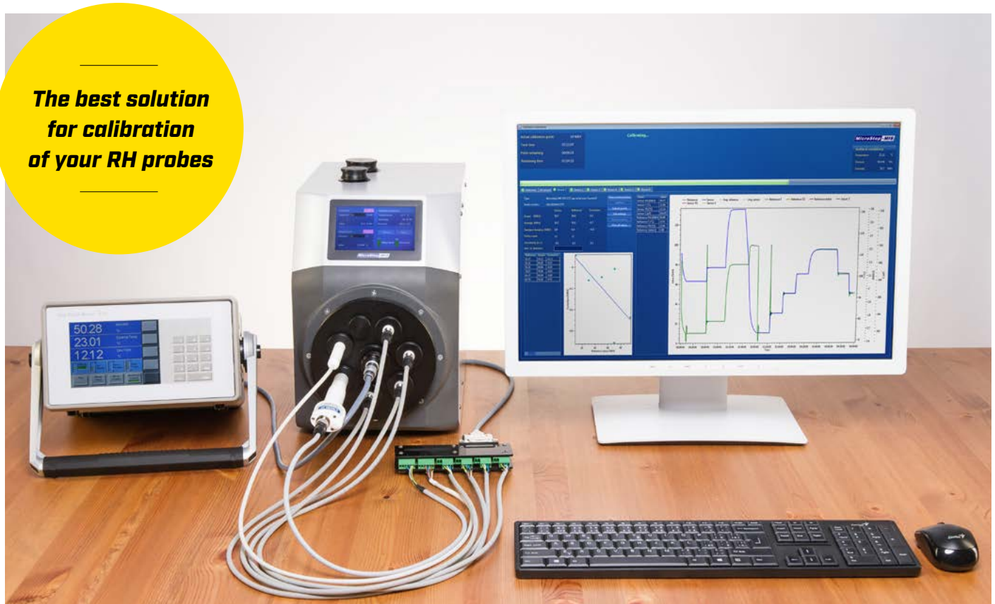
Laboratory workstation for Relative Humidity Calibration with Humiwell and dew point reference instrument
