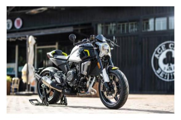
The engine produces a claimed 55kW (73hp) 8500rpm and 68Nm at 6500rpm, and other technical highlights include Bosch fuel-injection, split connecting rods, a slipper clutch and forged pistons for extra strength and reduced weight and inertia.
