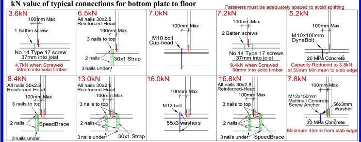
Wall frames manufactured by Wadsworth must be installed in accordance with AS1684-2010 and specific details provided.
