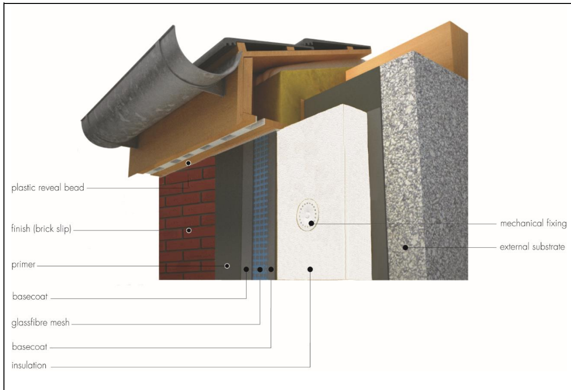
Figure 8 Roof eaves detail
