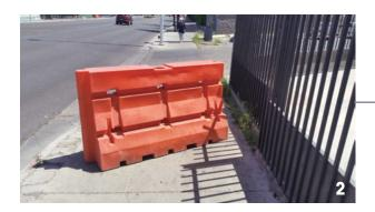
Water filled barriers rarely will disable let alone stop a vehicle at impact, are not an all-weather solution, require tankers to fill and are not mobile. They require exceedingly large amounts of space to store and may cause delays in emergency vehicle ingress/egress.
