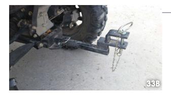
ATV hitch (rp-x18) mounted to ATV.
