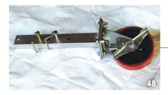
Castor assembly for K-2300sd barrier.
