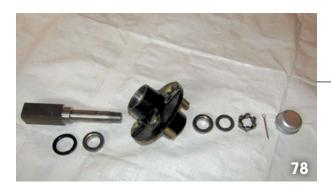
Replacement hub, spindle, bearings, seal, nut, dust cap, cotter pin, assembly for hd 208 transport kit.
