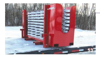
Four fork pocket rack positioned sideways on flat bed trailer.
