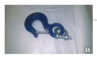
Slip hook with snap and clevis assembly.
