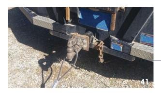
Potential cable anchoring point-- attached to the hitch of a truck. Site specific evaluations must be made in terms of potential attack speeds, surface types (where screw anchors cannot be installed-such as concrete streets etc.), aesthetic concerns, size of anchoring vehicle and anchoring vehicle footprint, and other considerations.
