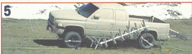
5 K2300, pick-up, unanchored, turf
