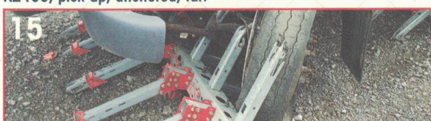
15 K2600 after ASTM impact
