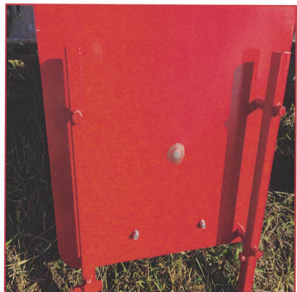
Back side of ballistic shield showing no full penetration nor pierce mark.
