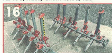
16 K2600 after ASTM impact barrier condition
