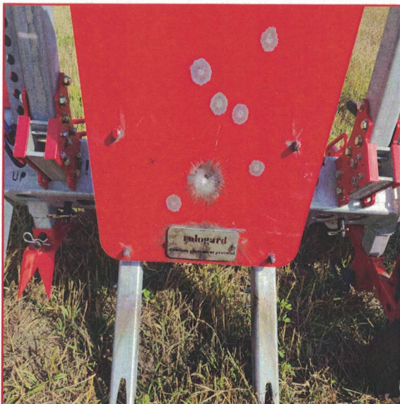
Rologard ballistic shield successfully stopped the round; same shield as the AR15 6 rnd volley.
