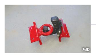
75mm pintle ring and latchable hook arrangement, hardware.
