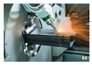
Virtual/real time manufacturing of our k2400hd splaying spar components, assuring the highest precision+produced efficiently-on the Trumpf TruLaser 7000 tube laser. It's fast and clean.
