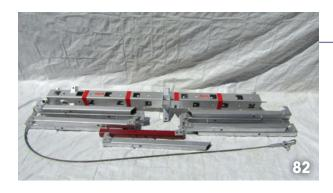
Disassembled base unit (hd200). Maximum single piece weight: 35.2 kgs
