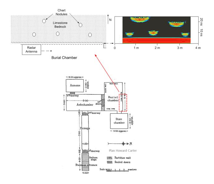
Figure 6: A simulation of a bedrock wall with chert nodule inclusions.
