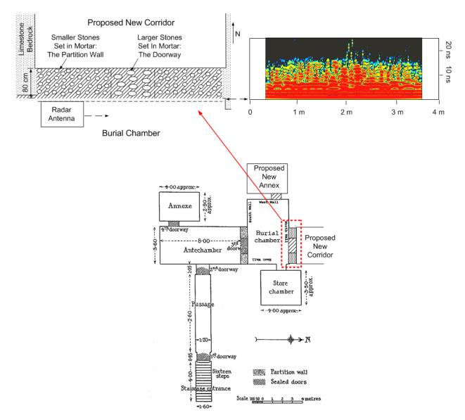
Figure 5: At the upper left is a sectional drawing of the wall Reeves suggests may separate the burial chamber from a hidden corridor. At the upper right is its simulated radar image.
