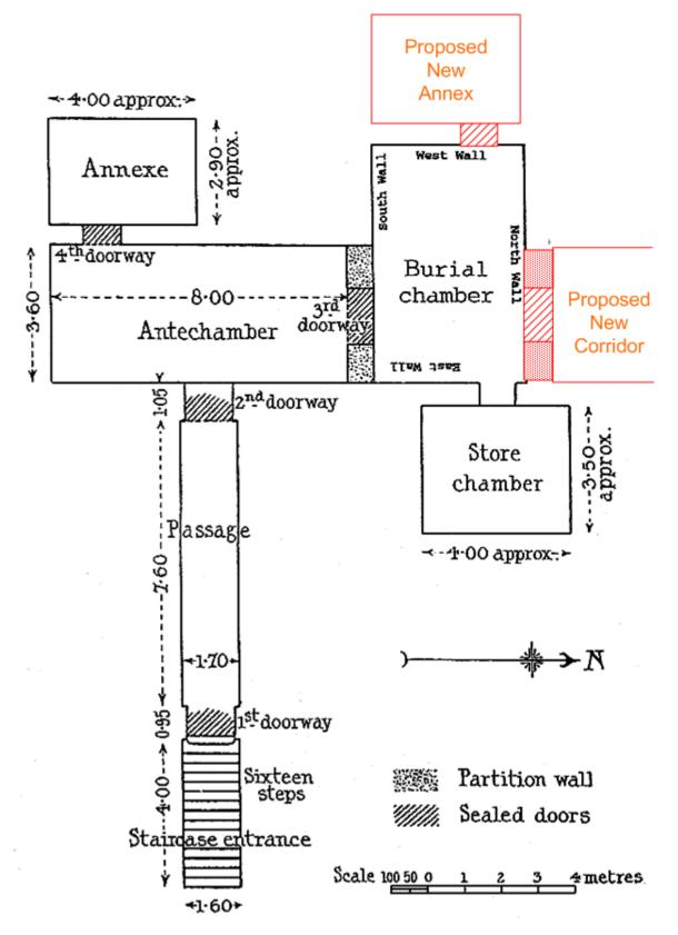
Figure 2: Carter's plan of the tomb of Tutankhamen with the proposed new annex and new corridor added. (Carter and Mace 1963, 223, with additions)
