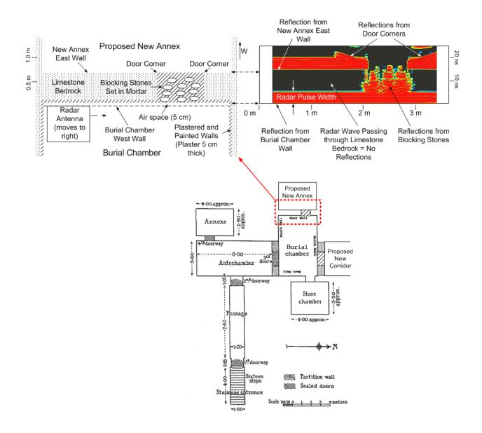
Figure 4: At the upper left is a "sectional" drawing of the wall (that is, a cut away view of the wall) that Reeves suggests stands between the burial chamber and the proposed new annex. At the upper right, a simulated radar image of the same section.
