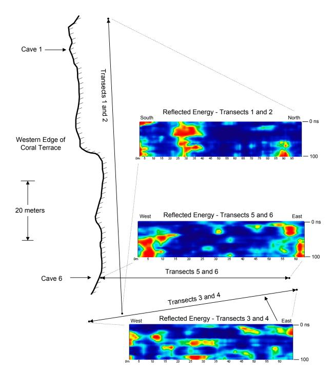
Figure 21: The map of reflected energy for these three pairs of transects shows areas where the rock is less homogeneous and therefore more reflective. This heterogeneity is likely caused by the movement of water from the top of the terrace either downward or preferentially across certain soil layers.
