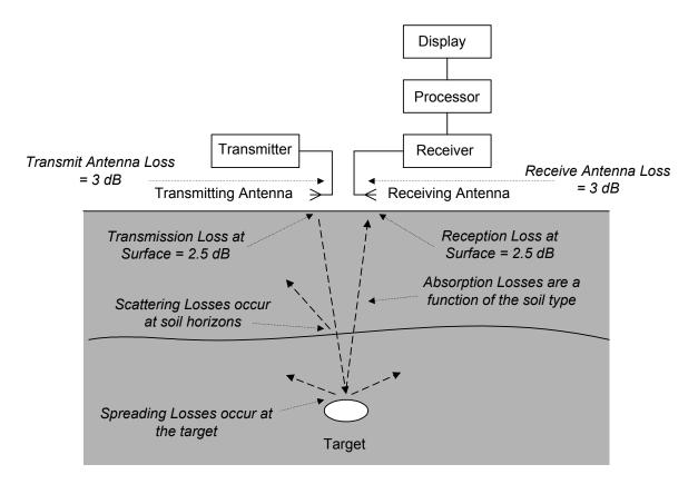
Figure 2: Losses which must be considered in predicting whether Ground Penetrating Radar will work in a given application.
