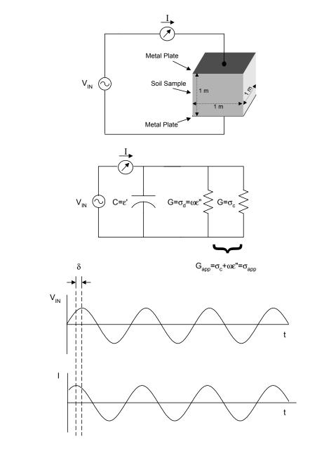
Figure 25: Conductivity, permittivity and phase. The phase delay  $\delta$  and the ratio of the current I to the voltage  $V_{IN}$  are used to derive the material's apparent conductivity and permittivity.
