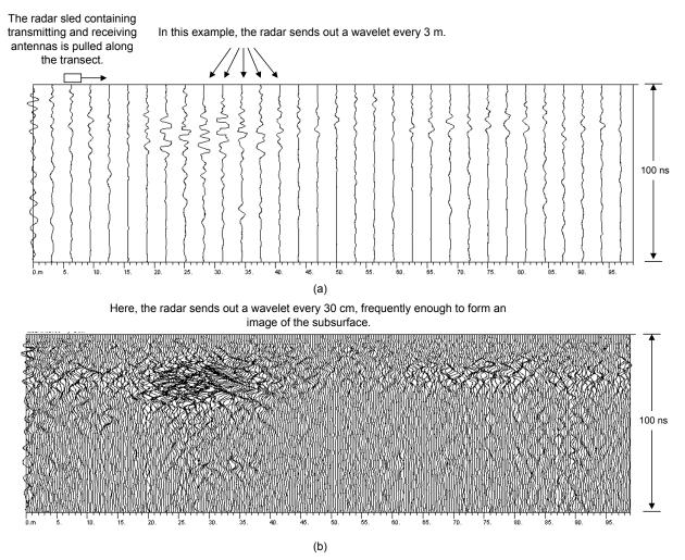
Figure 17: We record a subsurface radar profile by dragging a radar sled along a predetermined pathway. The radar can be adjusted to transmit a radar pulse, or wavelet, at intervals as it is dragged along. We record the received signal, or trace, at each location. At the top (a), the interval between transmissions is about 3 meters. At the bottom (b), the interval is reduced to about 30 cm and an image begins to form.
