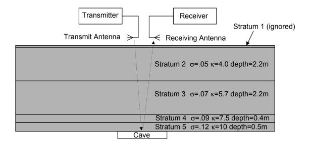
Figure 7: A simplified model of the strata at Mersa/Wadi Gawasis. The radar signal travels through a thin surface layer (which is ignored in the analysis) and four subsurface layers of varying properties. It reflects off the air-filled cave and returns to the surface.
