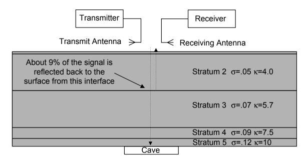
Figure 8: Velocity changes cause reflections. The change in velocity of the radar signal between Stratum 2 and 3 causes a reflection from their interface.
