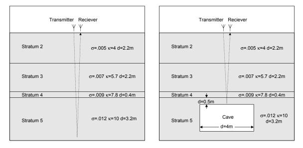
Figure 13: To use an electromagnetic wave simulator such as GprMax2D, we construct models of the volume we want to simulate. We have constructed two such volumes, one with and one without the cave.
