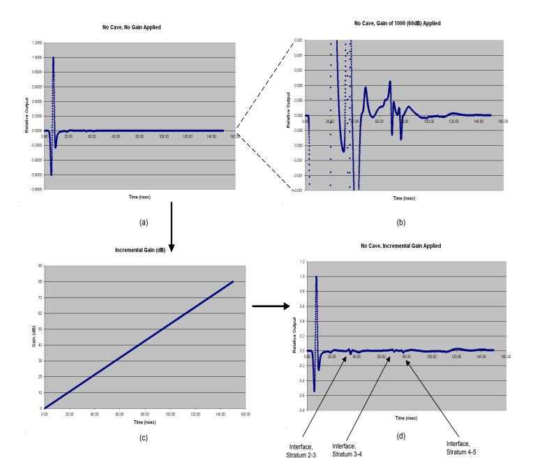
Figure 14: We show the output provided by GprMax2D without the cave present at (a). In order to see the reflections, we need to provide gain. We do so at (b) by magnifying the area around the x axis, effectively applying a gain of 1000. However, to better see the results, it is best to apply a gain that increases with time. The gain curve at (c) is applied to the plot at (a) to produce the result at (d).
