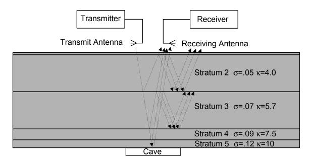
Figure 9: A more complete model of losses will include reflections from interfaces. When we include multiple reflections the model becomes computationally complex
