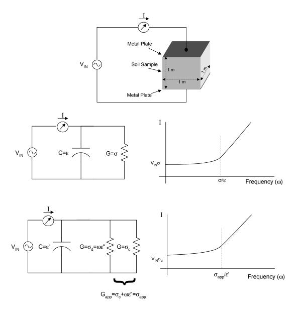
Figure 24: Conduction and dielectric currents. In a simplified model, current is dominated by conductivity (σ) at low frequencies and permittivity (ε) at higher frequencies. A more complete model includes dielectric losses.
