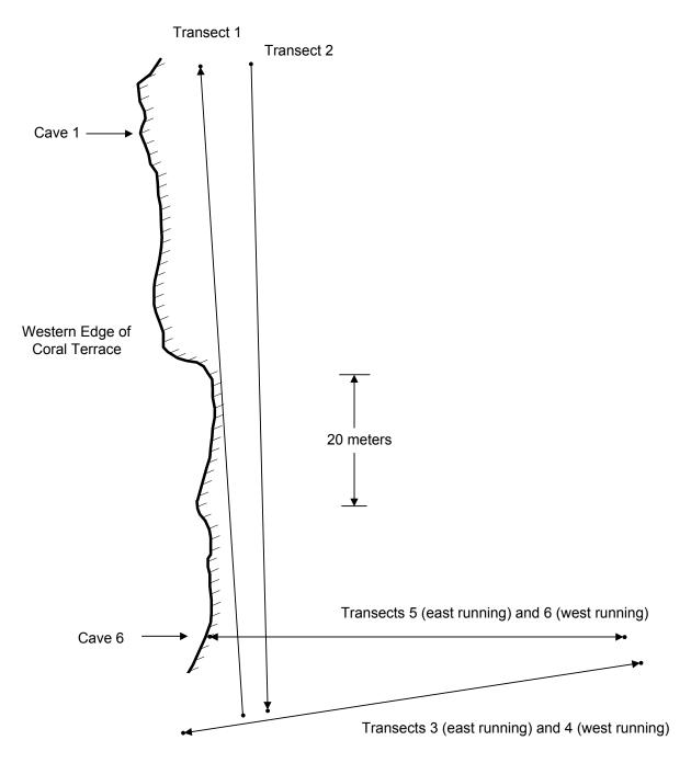
Figure 16: During a 2006-2007 field season, Mr. Benjamin Vining conducted radar surveys along six transects near the western edge of the coral terrace. Transects 1 and 2 ran south and north. Transects 3 and 4 ran roughly east and west. Two more east-west transects, 5 and 6, were run just to their north. (Credit: Vining 2006-2007)
