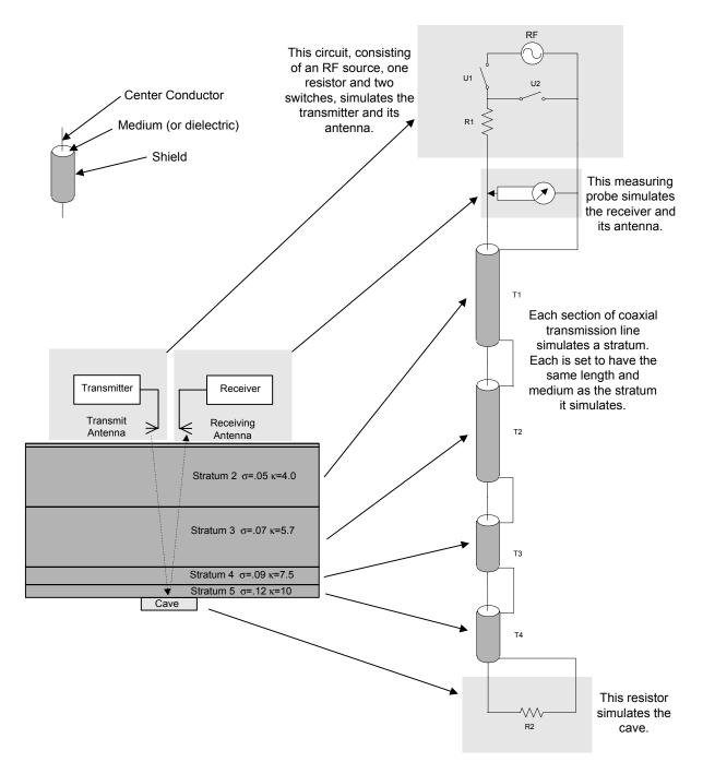
Figure 10: We can use PSPICE to predict scattering losses. Each stratum is modeled with a section of transmission line filled with a medium having the same properties as the soil we found at Mersa/Wadi Gawasis. The cave is simulated by a resistor. A combination of two switches, a resistor and a probe simulates the transmitter, receiver and their antennas.
