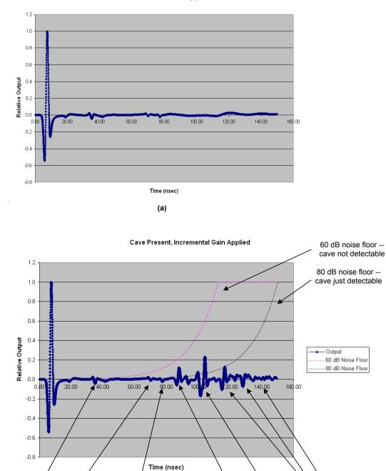
Figure 15: We show results without the cave present (a) and with the cave present (b). We applied incremental gain (Figure 14(c)) to the output of our simulation to create both traces. Whether the cave will be detectable depends on the noise floor. The dotted lines in (b) demark the 60 dB and 80 dB noise floors.
