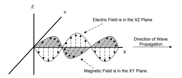
Figure 11: A propagating electromagnetic wave has two components: an electric field and a magnetic field, oriented at right angles to each other. The ratio of the amplitudes of the two fields is equal to the wave impedance.
