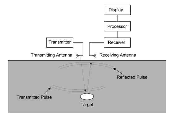
Figure 1: Block diagram of a Ground Penetrating Radar system.
