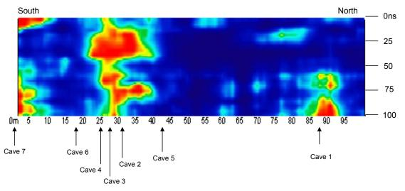
Figure 20: The reflected energy profile along north-south Transects 1 and 2 correlates well with the locations of Caves 1, 2, 3, 4 and 7.
