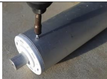
Install Small 95mm end slug
