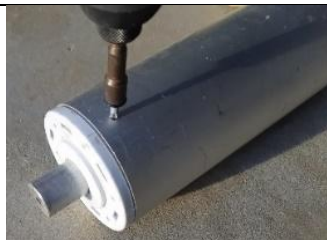
Install Small 95mm end slug
