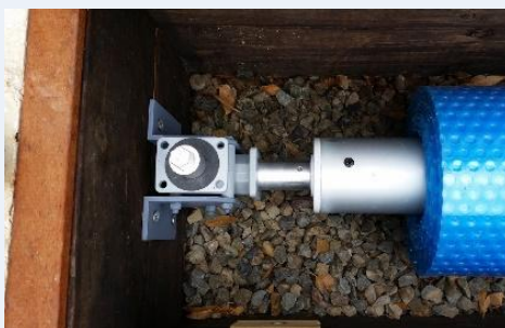
Roller tube mounted to gearbox
