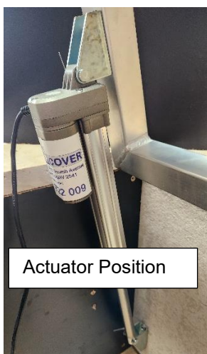
Acuator mounted on outside edge of Lid Frame
