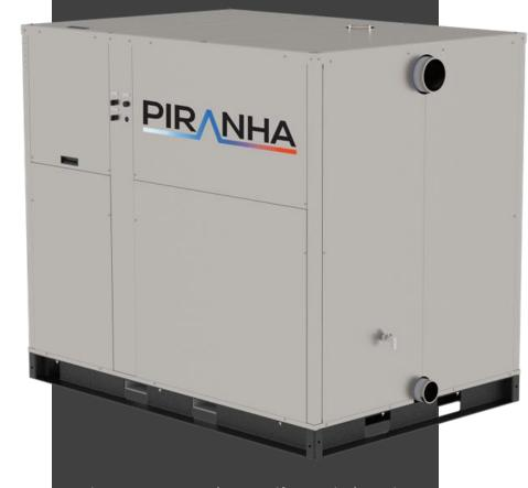
The PIRANHA is a self-contained heat pump that uses a specifically designed direct expansion heat exchanger to recover thermal energy from a building's wastewater for domestic hot water heating
