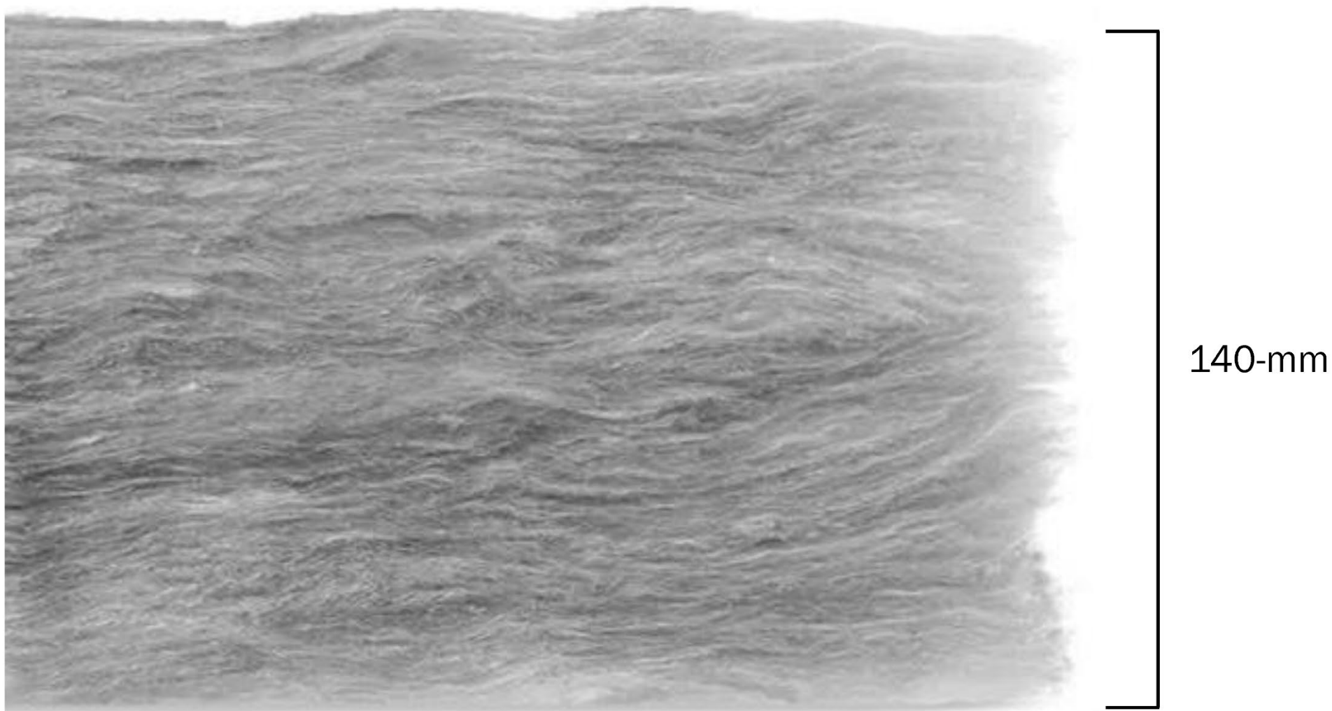
Fiberglass Insulation. R-18.
