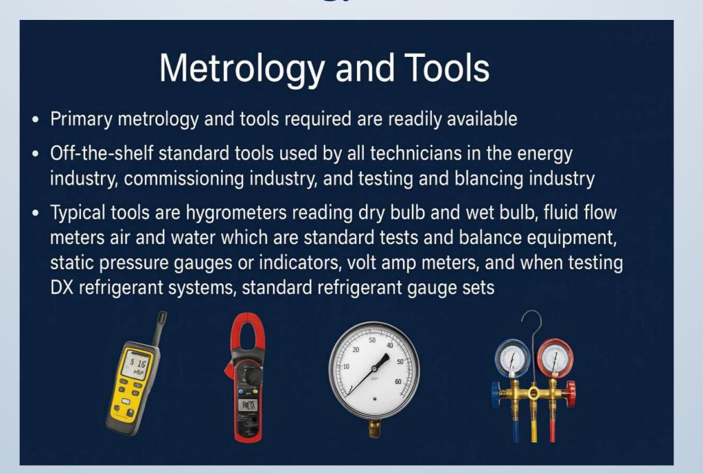
AMP uses standard, off-the-shelf field instruments, hygrometers, fluid flow meters, static pressure gauges, volt/amp meters, refrigerant gauges, tools every technician in the industry already knows. We integrate this with a software-directed process that eliminates inconsistencies and ensures precise performance verification.
