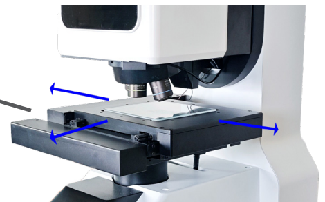
Motorized XY stage with travel range of 100mm x 100mm Repeatability: \leq \pm 1.5 \mu\text{m} Resolution: \leq 0.5 \mu\text{m} ax Max speed: \leq 30 \text{mm/s}
