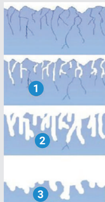
Operating principle of chemical etching in 3 steps.
