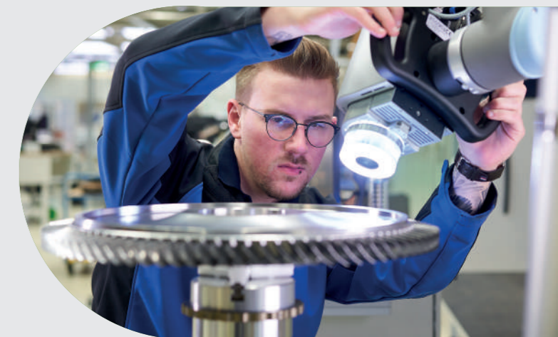
The operation of the Cobots is designed for the use of several operators. Handling, measurement and evaluation by means of programmed test routines are easy to handle, as MTU confirms.
