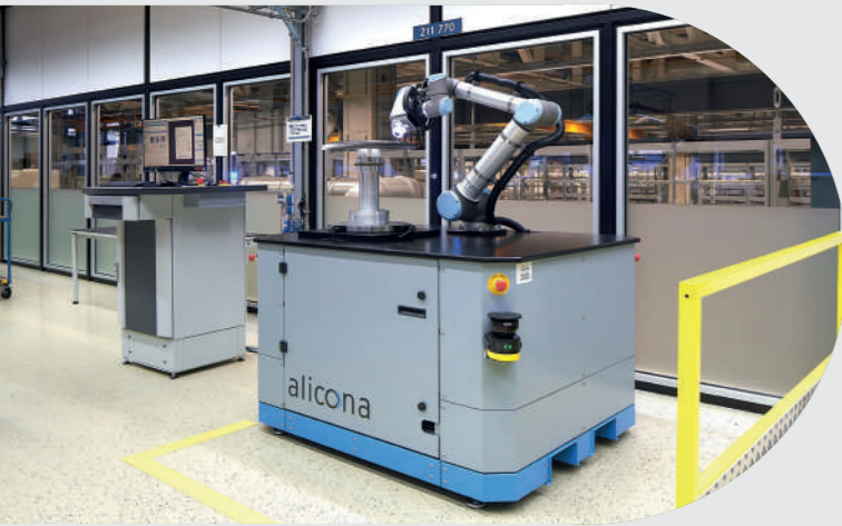
Cobots consist of a collaborative 6-axis robot and a high-resolution optical 3D measuring sensor and are a popular measuring device for production-integrated quality assurance.
