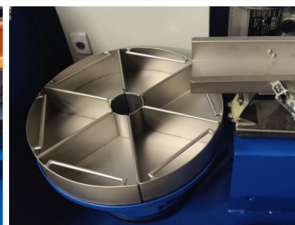
Rotary sample divider 6 x 16,6% bucket with custom grip point and height
