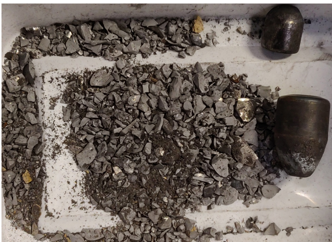
Tungsten carbide buttons processed by the LMFC250 Fine Crusher
