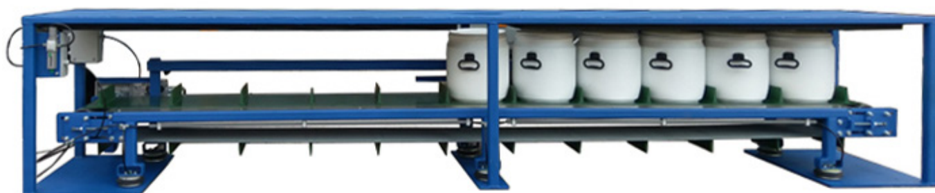
sample collector: straight conveyor
