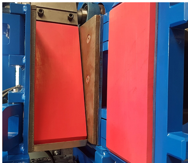
LMC100D Jaw Crusher with custom PU jaw plates
