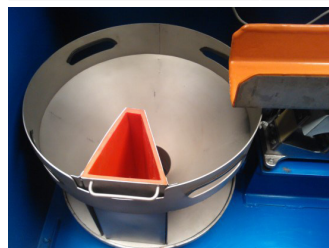
PU coating bucket and feeder
