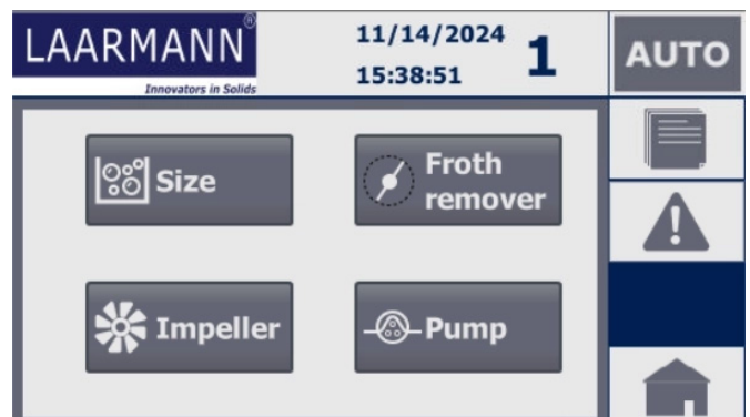
Flotation machine control panel interface
