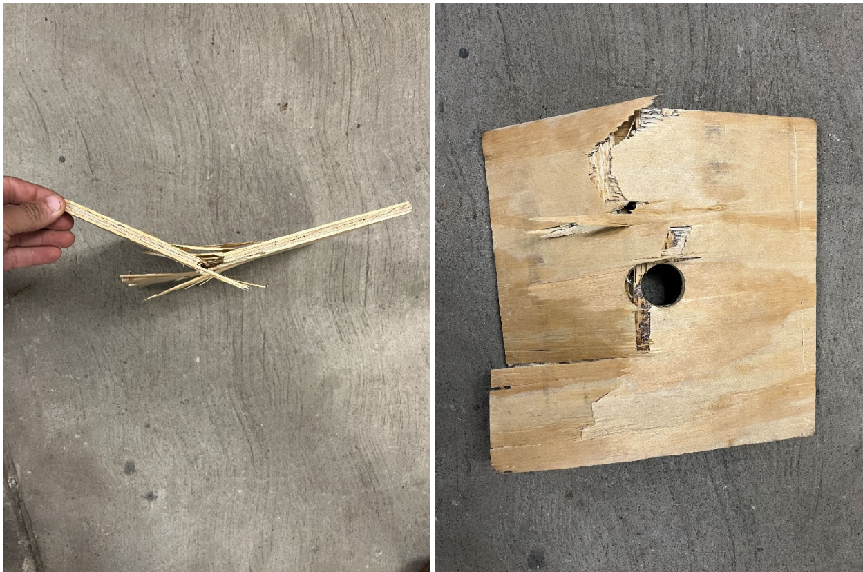
FIGURE 2.—Typical failure governed by bending with localized cracking and separations at the center of the plate near the applied load.
