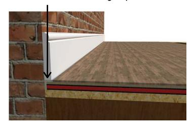
**T&G Engineered wood flooring** - Typically 14mm or thicker can be installed directly on top without the use of an additional stabilising layer but please check with your flooring supplier that the flooring is suitable for use a floating floor finish,
