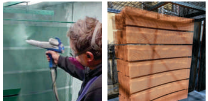
LEFT: Custom Gutter Guard screens that were manufactured for a commercial property being coloured post expansion.
