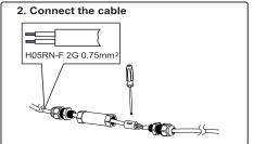
3. Tighten the cable by hand
