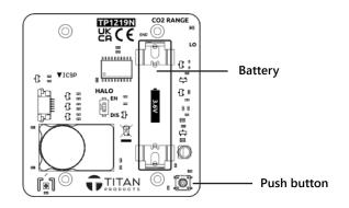
The sensors are supplied with a battery tab in place. Remove this before attempting to commission the device.
