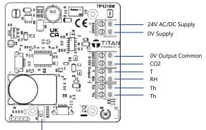
The HALO LED can be turned on/off using the switch
